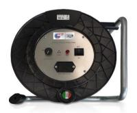
This level meter is used to measure the level of groundwater inside open tube piezometers, Casagrande piezometers, irrigation wells, and to measure the water level waterways, lakes and reservoirs. It is composed of a plastic reel mounted on a steel frame. The graduated signal cable is wrapped on the reel and it can be either round or flat. The stainless steel tip is attached to the
