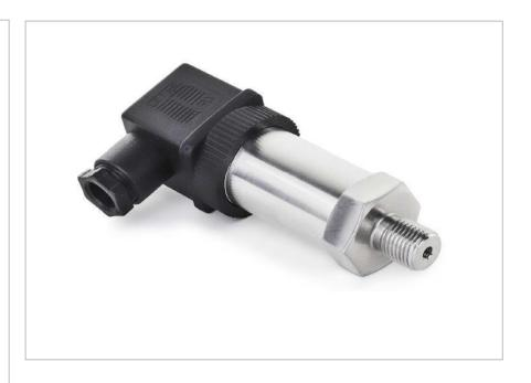
The industrial pressure transmitter is a transmitter used in pressure measurement for gases and liquids. It is designed with a stainless steel structure and has an internal digital circuit that can convert the millivolt signal of the sensor into a standard voltage or current signal output.
