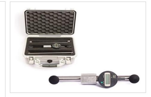
The mechanical deformometer is a measuring tool to assess changes in the distance (relative displacement) between two reading bases with order of magnitude of one thousandth of a millimetre.
